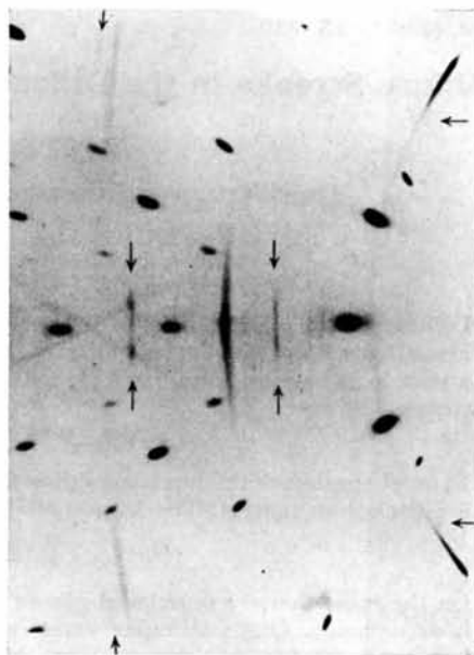
Fig. 1. Four pairs of diffuse streaks on a Laue-photograph taken from a common specimen. The long arcs are vanadium powder lines due to disturbed surface layers. Axis [001]_{\text{b.c.c.}} parallel to the vertical axis of the goniometer. Glancing angle i_{100} = 30^\circ 33' .
